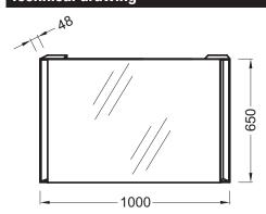
Product Specification: Mirror 100 cm. EB576. Collection:  $R\hat{E}VE$ . Dimensions:  $100 \times 5 \times 65$  cm. Weight: 13.8 kg. Installation: Wall-mount. Power: 230 V,  $2 \times 24 \text{ W}$ , 74 fitting, class II, IP44, energy efficiency class A. Note: the infrared sensor switch requires a gap of at least 15 cm between itself and the tile or other object.
