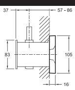
Product Specification: Bath filler. 922W. Collection: LAMINAR. Installation: Wall-mount. Flow rate: 19-38 l/min. Wall or ceiling mounted. 20 mm opening.
