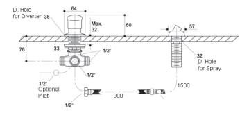
Product Specification: Diverter valve, incl. hand shower hose guide. 8549. Collection: LAMINAR.
