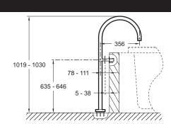
Product Specification: Floor-mount bath spout. 8359W. Collection: LAMINAR. Weight: 6.3 kg. Installation: Floor-mount. Flow rate: 43 I/min. Flow rate: 43 I/min. Floor.
