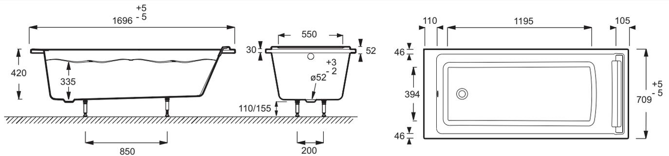
Product Specification: Bath 170 x 70 cm. 6D009. Collection: SPACIO. Dimensions: 170 x 70. Weight: 23 kg. Material: Acrylic. Installation: Drop in. Volume: 217. Adjustable feet. Neck support.
