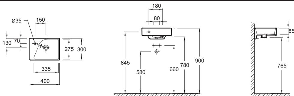
Product Specification: Handwash basin 40 cm. 5091K. Collection: FORMILIA. Dimensions: 40 x 30. Weight: 9.2 kg. Material: Ceramic. Installation: Self-supporting or can be mounted on a specific cabinet. Faucet drilling: 1 faucet hole. Asymmetrical shape and dynamic lines. Chromed overflow cap.
