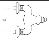
Product Specification: Single-lever wall-mount shower mixer. 19563D. Collection: FAIRFAX. Weight: 1.5 kg. Installation: Wall-mount. Flow rate: 20 l/min. Flow rate: 20 l/min. Connection: With connectors and wall escutcheons. Mechanism: Ceramic disc cartridge. Hole configuration: 150 mm. Retro style with a modern touch on a single-lever mixer. Non-return valve on shower outlet. Temperature limiter ring.
