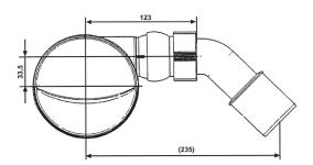
Product Specification: Drain for shower tray Ø 6 cm. 19199. Collection: NO COLLECTION. Weight: 0.2 kg. Flow rate: 45 l/min.
