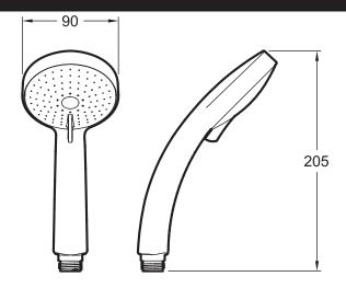
Product Specification: 4-spray handshower Ø 90 mm. 12902D. Collection: CITRUS. Weight: 1 kg. Flow rate: 9.5 l/min. Anti-scale system. Flow control.
