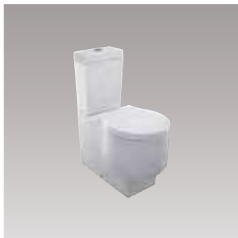
Viragio back-to-wall WC pan with cistern 64 x 36.5 cm vario outlet with slow-close seat comfort height 41 cm low flush 2.6/4 L or 3/6 L possible 4449K + 4790K/4443K
