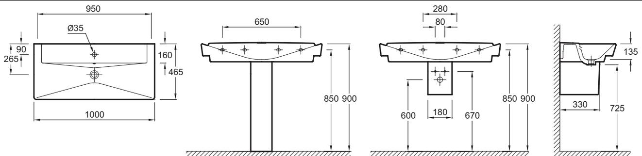
Product Specification: 1-hole vanity top 100 cm. 5026K. Collection: RÊVE. Dimensions: 100 x 46.5. Weight: 34.3 kg. Material: Ceramic. Installation: Self-supporting. Can be mounted onto specific cabinet, with or without pedestal/semi-pedestal/shroud. Faucet drilling: 1 central faucet hole. Wide ledge for optimal comfort of use. Combination of straight lines and softened angles. Perfect fit with cabinet. Without overflow 5086K. With 3 tap holes 5026K-8. Chromed overflow cap.
