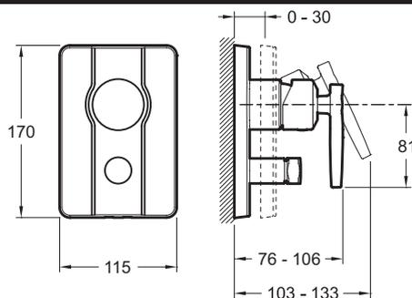
Product Specification: Trim and lever for built-in bath/shower mixer. E98725. Collection: MODULO. Flow rate: 30 l/min. / 25 l/min.. Incl. single-lever built-in mixer. Automatic diverter with locking option. Incl. non-return valve. Ceramic disk cartridge. DVGW NW-6512CP0428.
