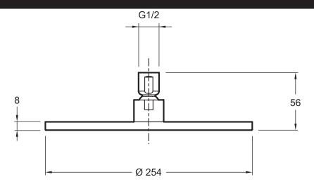
Product Specification: Round metal showerhead Ø 25 cm. 14568D. Collection: EO. Weight: 1.4 kg. Flow rate: 10 I/min. In metal with anti-scale system. Extra slim (8 mm). to be mounted on the wall or ceiling. Large coverage: 250 mm. Flow rate: 10L/min.
