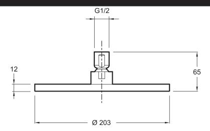
Product Specification: Round metal showerhead ø 20 cm. 14536D. Collection: E0. Weight: 1.7 kg. Flow rate: 10 l/min. In metal with anti-scale system. To be mounted on the wall or ceiling. Flow rate: 10L/
