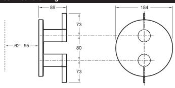
Product Specification: Thermostatic shower trim. T10941-4. Collection: STILLNESS. Weight: 3.1 kg. Installation: Wall-mount. Steamlined element. pure design and industrial integrity lend aesthetic functionality to minimal spaces.
