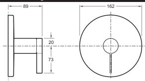
Product Specification: Thermostatic shower trim. T10940-4. Collection: STILLNESS. Weight: 2.9 kg. Installation: Wall-mount. Steamlined element. pure design and industrial integrity lend aesthetic functionality to minimal spaces.
