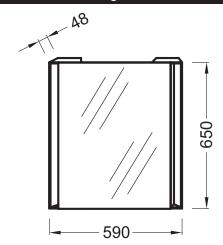
Product Specification: Mirror 60 cm. EB575. Collection: RÊVE. Dimensions: 59 x 5 x 65 cm. Weight: 12 kg. Installation: Wall-mount. Power: 230 V, 2 x 24 W, T4 fitting, class II IP44, energy efficiency class A. Note: the infrared sensor switch requires a gap of at least 15 cm between itself and the tile or other object.
