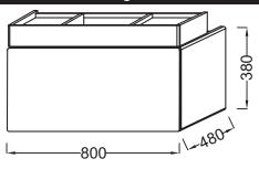
Product Specification: Base unit 80 cm. EB1186. Collection: TERRACE. Dimensions: 80 x 48 x 38 cm. Weight: 28 kg. Material: Lacquer. Installation: Wall-hung. 1 lacquered push release drawer. 1 solid wood accessoires drawer with push release.
