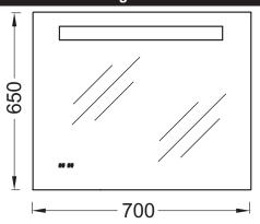
Product Specification: Mirror 70 cm, with lighting and digital clock. EB1159. Collection: MIRRORS. Dimensions: 70 x 3 x 65 cm. Weight: 9.7 kg. Installation: Wall-mount. Power: 230 V, 7 W, class II, IP44, energy efficiency class A++. Digital clock. Anti-steam feature. Infrared sensor switch located below the mirror. LED lighting: 230 V, 7 W, class II, IP44, energy efficiency class A++. Note: the infrared sensor switch requires a gap of at least 15 cm between itself and the tile or other object.
