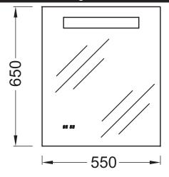
Product Specification: Mirror 55 cm, with lighting and digital clock. EB1158. Collection: REPLAY. Dimensions: 55 x 3 x 65 cm. Weight: 7.9 kg. Installation: Wall-mount. Power: 230 V, 5 W, class II, IP44, energy efficiency class A++.
