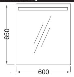
Product Specification: Mirror 60 cm, with lighting. EB1151. Collection: NO COLLECTION. Dimensions: 60 x 3 x 65 cm. Weight: 7.7 kg. Installation: Wall-mount. LED lighting: 230 V, 6 W, class II, IP 44. Infrared sensor switch.
