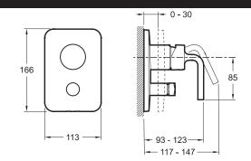
Product Specification: Trim and lever for built-in bath/shower mixer. E98721. Collection: PURISTIC. Incl. single-lever built-in mixer. Automatic diverter with locking option. Incl. non-return valve. Ceramic disk cartridge. DVGW NW-6512CP0428.
