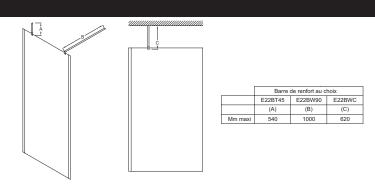
Product Specification: Vertical bracing bar. E22BWC. Collection: CONTRA. Attached to ceiling.
