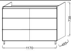
Product Specification: Base unit 117 cm. 99381K. Collection: REACH. Dimensions: 117 x 48.5 x 74 cm. Weight: 62 kg. Material: Solid color decor or wood decor. Installation: Raised.
