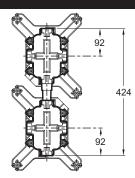
Product Specification: Box connector to align 2 superposed boxes. 98788D. Collection: MODULO. Installation: Built-in. Install to connect two Modulo universal boxes 98699D-NF. Easier alignment of two boxes. perfect esthetics. Better seal between the two boxes.
