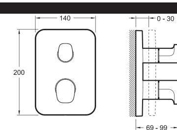
Product Specification: Hybrid trim for built-in bath/shower mixer. 98730D. Collection: MODULO. Installation: Wall-mount. Incl. thermostatic and flow-control valve. Instantaneous water heater suitable. Filter and non-return valves. DVGW NW-6512CP0430.
