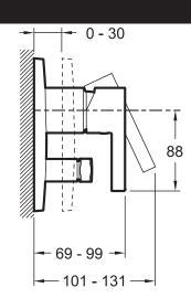
Product Specification: Trim and lever for built-in bath-shower mixer. 98723D. Collection: STANCE. Installation: Wall-mount. Incl. single-lever built-in mixer. Incl. non-return valve. Automatic diverter with locking option. Ceramic disk cartridge. DVGW NW-6512CP0428.
