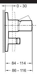
Product Specification: Trim and lever for built-in bath-shower mixer. 98719D. Collection: CÜFF. Weight: 2.5 kg. Installation: Wall-mount. Normes: ACS (Certificate of Sanitary Compliance): 10 ACC LY 004. Incl. single-lever built-in mixer. Incl. non-return valve. Automatic diverter with locking option. Ceramic disk cartridge. DVGW NW-6512CP0428.
