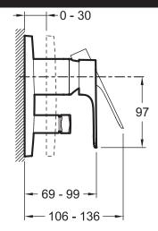
Product Specification: Trim and lever for built-in bath/shower mixer. 98718D. Collection: ALEO+. Installation: Wall-mount. Mount with Modulo universal box 98699D-NF. Kit composed of built-in body. trim. handle and diverter. Easy-to-install cartridge. thanks to guide notches. Automatic diverter with locking option. Non-return valve.
