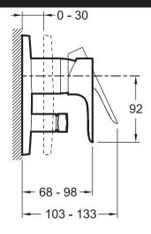
Product Specification: Trim and lever for built-in bath/shower mixer. 98717D. Collection: ALEO. Installation: Wall-mount. Mount with Modulo universal box 98699D-NF. Kit composed of built-in body. trim. handle and diverter.
