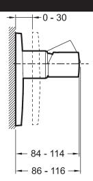
Product Specification: Trim and lever for built-in shower mixer. 98707D. Collection: CÜFF. Weight: 1.9 kg. Installation: Wall-mount. Normes: ACS (Certificate of Sanitary Compliance):10 ACC LY 004. Incl. single-lever built-in mixer. Incl. non-return valve. Ceramic disk cartridge. DVGW NW-6512CP0427.
