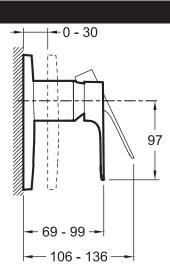
Product Specification: Trim and lever for built-in shower mixer. 98706D. Collection: ALEO+. Installation: Wall-mount. Mount with Modulo universal box 98699D-NF. Kit composed of built-in body. trim. handle and diverter. Easy-to-install cartridge. thanks to guide notches. Ceramic disk cartridge.
