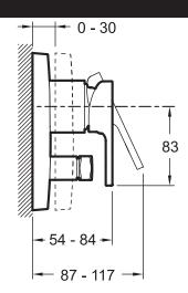
Product Specification: Trim and lever for built-in bath/shower mixer. 98633D. Collection: MODULO. Weight: 2.9 kg. Installation: Wall-mount. Normes: ACS (Certificate of Sanitary Compliance): 10 ACC LY 004. Incl. single-lever built-in mixer. Incl. non-return valve. Ceramic disk cartridge. DVGW NW-6512CP0428.
