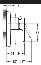
Product Specification: Trim and lever for built-in shower mixer. 98632D. Collection: MODULO. Weight: 2.1 kg. Installation: Wall-mount. Normes: ACS (Certificate of Sanitary Compliance): 10 ACC LY 004. Incl. single-lever built-in mixer. Incl. non-return valve. Ceramic disk cartridge. DVGW NW-6512CP0427.
