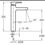
Product Specification: Tall single-lever washbasin mixer. 98340D. Collection: STRAYT. Installation: 1 hole. Flow rate: 5 l/mn. Ceramic disc cartridge. Incl. pop-up drain. Water saving feature. Anti-scale aerator.
