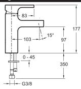
Product Specification: Single-lever washbasin mixer. 98339D. Collection: STRAYT. Installation: 1 hole. Flow rate: 5 I/mn. Ceramic disc cartridge. No drain. Water saving feature. Anti-scale aerator.
