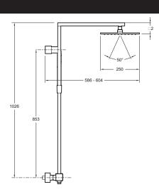
Product Specification: Thermostatic shower column. 98321D. Collection: STRAYT. Dimensions: 25 x 25 cm. Weight: 11.7 kg. Installation: Wall-mount. Shift Square 2-sprays handshower. FLOW RATE: Shower-FLOW RATE: S head 13 I/min, handshower 9.5 I/min.
