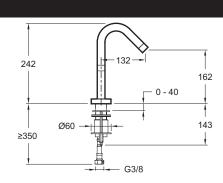
Product Specification: Single-lever washbasin mixer. 979D-4. Collection: STILLNESS. Weight: 1.9 kg. Installation: 1 hole. Flow rate: 6 l/min. Connection: With supply hoses. Mechanism: Sequential cartridge. Steamlined element. pure design and industrial integrity lend aesthetic functionality to minimal spaces. Anti-scale system. No lift rod.
