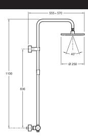
Product Specification: Thermostatic shower column. 8993D. Collection: TOOBI. Dimensions: Ø 25 cm. Weight: 8 kg. Installation: Wall-mount. Shift Ellipse handshower 2 sprays. FLOW RATE: showerhead 101/ min., handshower 9.5 l/min.
