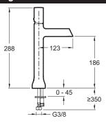
Product Specification: Tall single-lever washbasin mixer. 8960D. Collection: TOOBI. Weight: 1.6 kg. Installation: 1 hole. Flow rate: 8 l/min. Flow rate: 8 l/min. Connection: With supply hoses. Mechanism: Ceramic disc cartridge. Pop art inspiration. No waste. Flow limited to 8 l/min. 2 spout inserts (white and green) for personnalization.
