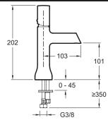
Product Specification: Tall single-lever washbasin mixer. 7329D. Collection: TOOBI. Weight: 1.3 kg. Installation: 1 hole. Flow rate: 8 l/min. Flow rate: 8 l/min. Connection: With supply hoses. Mechanism: Ceramic disc cartridge. No drain. Ceramic disc cartridge. Green. white and black spout inserts.
