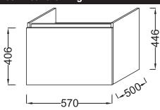
Product Specification: Base unit, 57 cm. 7276K. Collection: PARALLEL. Dimensions: 57 x 50 x 40.6 cm. Weight: 17 kg. Material: Solid color decor or wood decor. Installation: Wall-hung. Storage solutions to complete your made-to-measure washstation. Base unit with 1 slow-close drawer. With trap opening.
