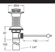
Product Specification: Basin remote pop-up drain -for basin without overflow. 7114. Collection: NO COLLECTION. Weight: 1 kg. For basin without overflow.
