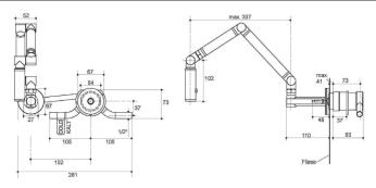
Product Specification: Articulating wall-mount kitchen faucet. 6228-C11. Collection: KARBON. Weight: 4.9 kg. Installation: Wall-mount. Flow rate: 6.8 l/min. Fixings: Wall-mount. Flow rate: 6.8 l/mi nism: Ceramic cartridge "joystick" type. 5 articulations for perfect mobility and positioning. 2 delivery options: Forceful spray and laminar stream.
