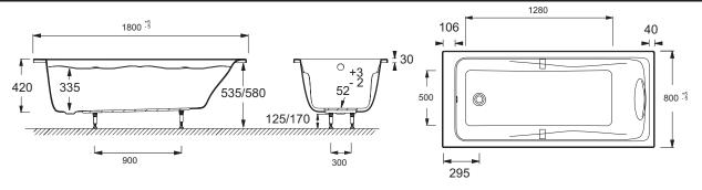
Product Specification: Whirlpool bath, Massdream system, 180 x 90 cm. 5BE2190. Collection: REACH. Dimensions: 200 x 100. Material: Acrylic. Installation: Built-in. Volume: 290. Massages type: Water massage. Jets: Back massage: 8 mini-jets. Safety system: Safety feature (no water). Invisible controls. 1 Waterfall pillow. Pump 900 W. Self-supporting frame.
