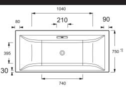
Product Specification: Whirlpool bath, Plus system, right handed, 170 x 75 cm. 5BB213R. Collection: EVOK. Dimensions: 170 x 75. Weight: 21 kg. Material: Acrylic. Installation: Built-in. Volume: 217. Massages type: 2 Massage programs (Silence and Tonic): water massages. Jets: Back massage: 4 mini-jets; Foot massage: 2 rotating jets; Body massage: 6 rotating jets. Safety system: Safety feature (no water). 3-button keypad. 1 LED spotlight. Pump 900 W. Self-supporting frame.
