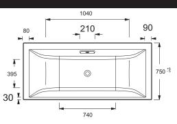
Product Specification: Whirlpool bath, Plus system, left handed, 170 x 75 cm. 5BB213L. Collection: EVOK. Dimensions: 170 x 75. Weight: 21 kg. Material: Acrylic. Installation: Built-in. Volume: 217. Massages type: 2 Massage programs (Silence and Tonic): water massages. Jets: Back massage: 4 mini-jets; Foot massage: 2 rotating jets; Body massage: 6 rotating jets. Safety system: Safety feature (no water). 3-button keypad. 1 LED spotlight. Pump 900 W. Self-supporting frame.
