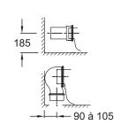
Product Specification: Independent back-to-wall WC pan 56 x 36, 5 cm. 5038K. Collection: RÊVE. Dimensions: 56 x 36.5. Weight: 36.7 kg. Material: Ceramic. Installation: Floor-standing. Toilet with contemporary lines. Slow-close thermoset seat E6402 and metal hinges included. Enhanced seating comfort: height 41 cm and ergonomic seat.
