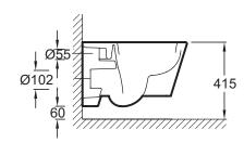
Product Specification: Wall-hung WC pan 56 x 36.5 cm. 5036K. Collection: RÊVE. Dimensions: 56 x 36.5. Weight: 26.5 kg. Material: Ceramic. Installation: Wall-hung. Toilet with contemporary lines. Slow-close thermoset seat E6402 and metal hinges included. removable. Water saving 3/6Ldual flush. The distance between the mounting holes is 230 mm.
