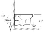
Product Specification: Wall-hung WC pan 54 x 36.5 cm. 4843K. Collection: REPLAY. Dimensions: 54 x 36.5. Weight: 26.9 kg. Material: Ceramic. Installation: Wall-hung. Fixings: Concealed fixings included. Soft. classic lines. Order toilet seat separately. Concealed fixings supplied. Low flush 2.6/4 L or 3/6 L possible. Perfect fit with Replay vanity tops and cabinets. Closed glaze rim.
